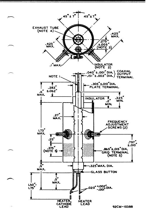
NOTE 1: THE AXES OF THE INNER AND OUTER CONDUCTORS OF THE COAXIAL OUTPUT TERMINAL COINCIDE WITHIN 0.010".
