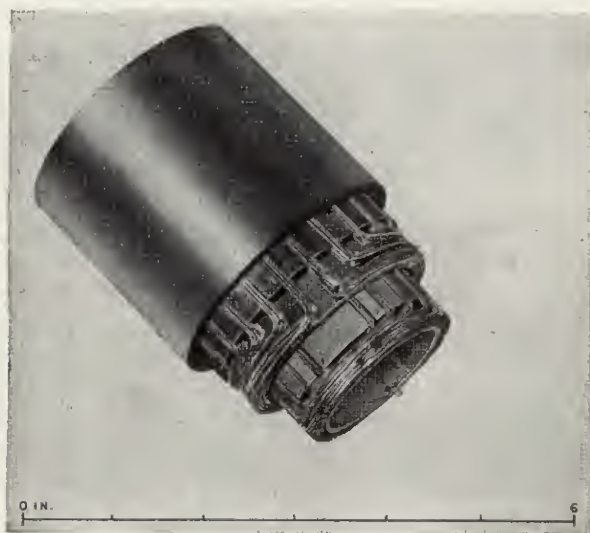
Fig. 8-30.—Compound deflection coil, extended to show construction.
