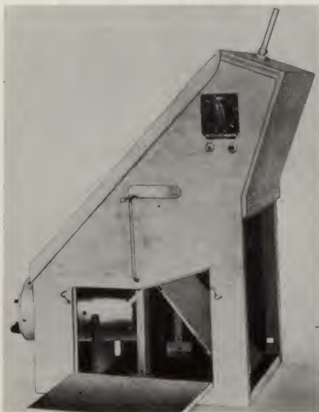
FIG. 18-74.—Detailed view of light-tight box for 931 phototube mount, red light, and lamp timer.
