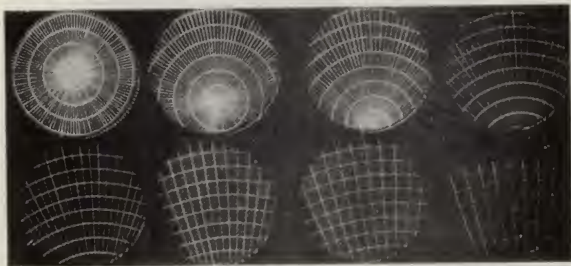
FIG. 12-14.—Radial-time-base display in various off-centered positions.
