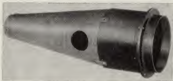
FIG. 16-1.—Support and magnetic shield for 5-in. electrostatic tube.
