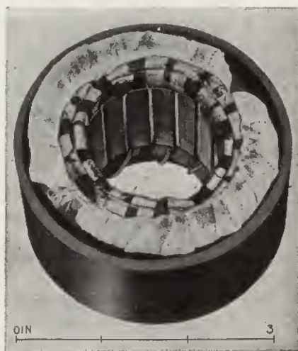
FIG. 8-31.—Motor-stator deflection coil wound for push-pull horizontal and vertical deflection.
