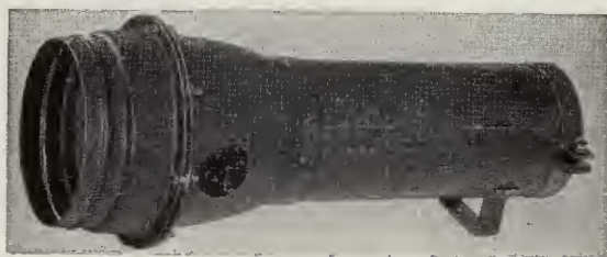
FIG. 16-2.—Tube mount and shield for 3-in. electrostatic tube.
