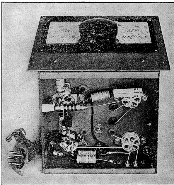
Fig. 1256 — High-frequency connections underneath the chassis of the v.f. exciter unit are made with short, straight sections of heavy wire. The two zero-temperature padding condensers are soldered directly to the oscillator-coil socket. All components are mounted firmly with no opportunity to support mechanical vibration. Washers \frac{1}{16} -inch thick are placed between the panel and the chassis to provide space for the lower lip of the cabinet opening.
