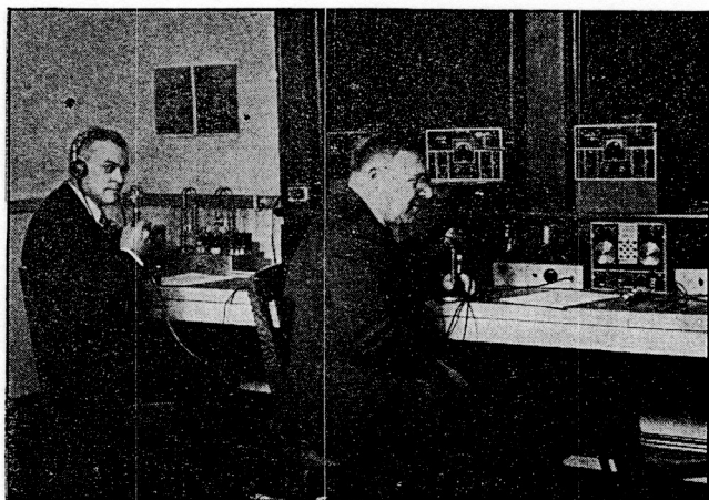
Fig. 1603 — A typical WERS district control center station — WODF-5, Akron, Ohio. Duplicate operating positions enable dual-channel contacts with the central control station and field groups simultaneously. Auxiliary transceivers are kept in reserve to supplement regular equipment in the event of failure and for use as field units.
