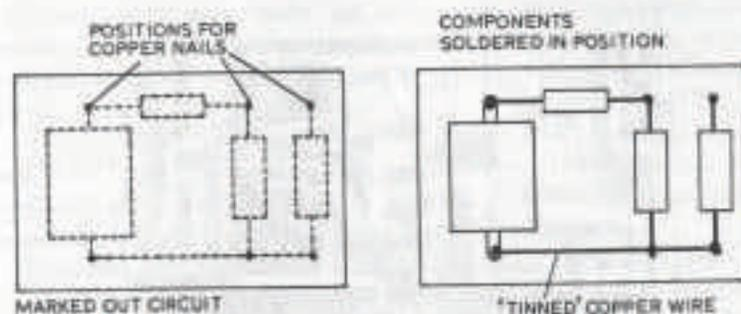
Fig. 12.6 'Copper nail' technique—again suitable for small circuits.
