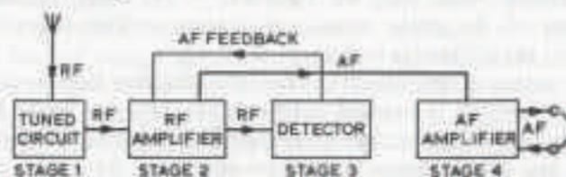
Fig. 9.4 Block diagram of a four-stage reflex receiver.
