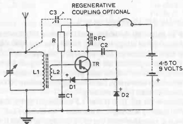
Fig. 9.8 *Circuit 19*. Single-transistor reflex receiver using two diodes.
