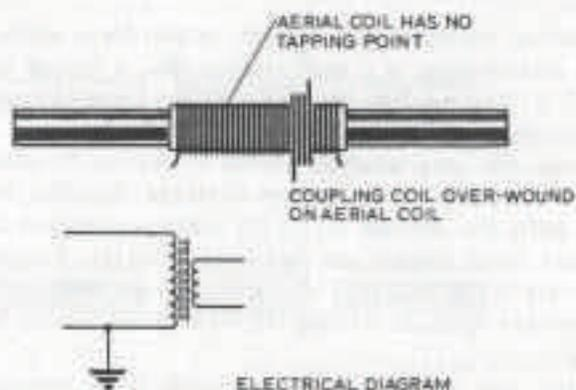
Fig. 4.5 Inductively-coupled aerial coil.
