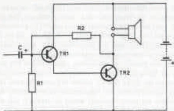
Fig. 5.4 Circuit 7. Amplifier for loudspeaker output
