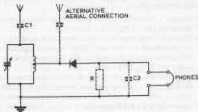
Fig. 3.5 Circuit I. Circuit diagram of basic crystal set.
