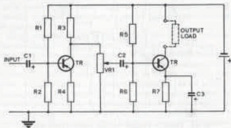
Fig. 5.7 Circuit 9. Two-stage amplifier with volume control.
