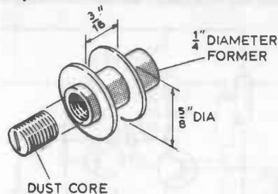
Fig. 9.7 Coil former for winding the RFC coils.
