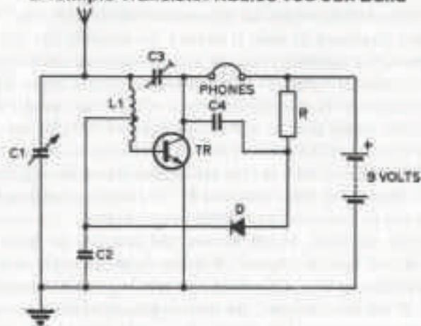
Fig. 9.5 Circuit 17. Single-transistor three-stage reflex receiver.
