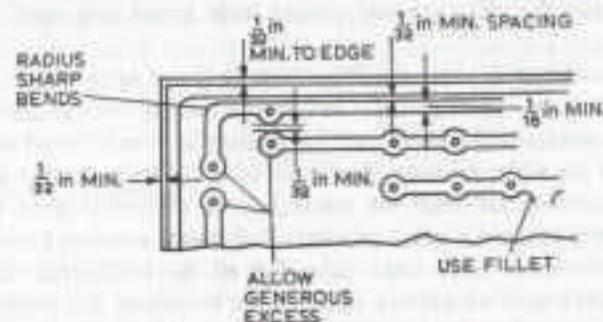
Fig. 12.9 Recommended proportions for conductors, spacing etc.
