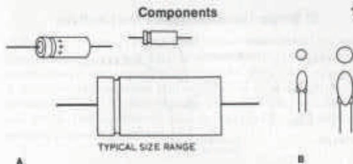
Fig. 11.9 Electrolytic capacitors
