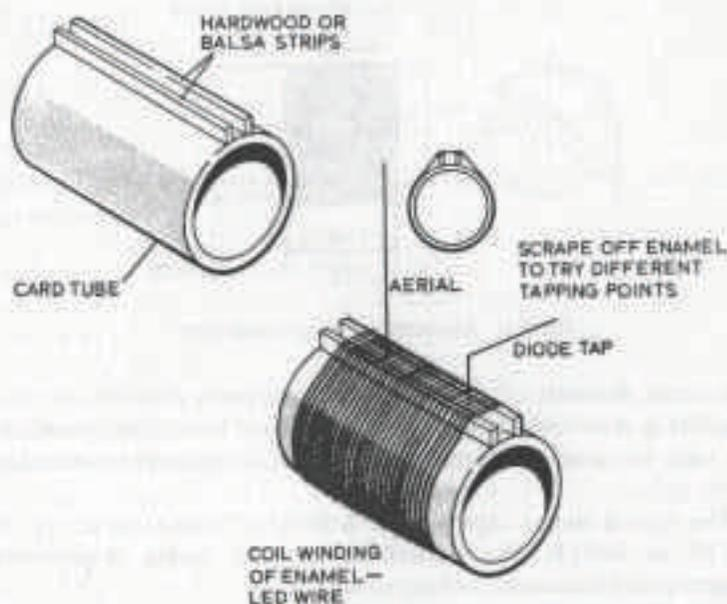
Fig. 4.3 Construction of an air-cored aerial coil.
