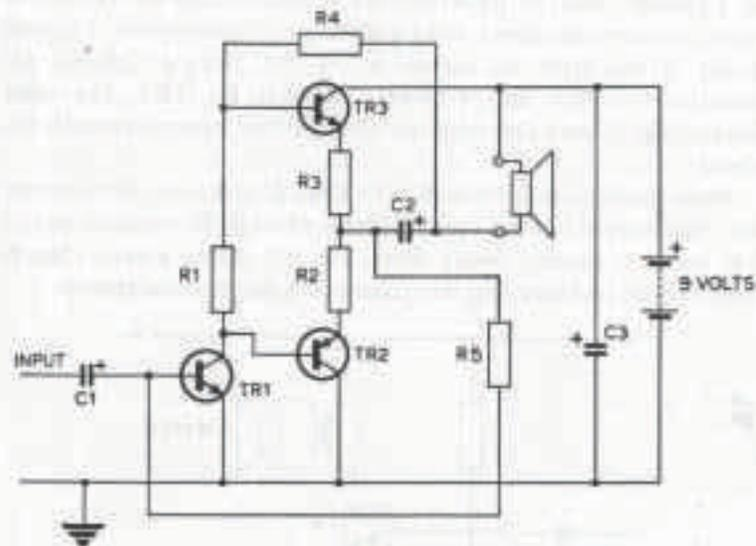
Fig. 6.2 Circuit 10. Push-pull output. TR1 is the driver, TR2, TR3 the push-pull amplifier.
