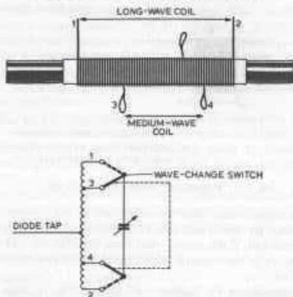
Fig. 4.7 Long- and medium-wave serial coil connected to wave-change switch.
