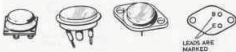
Fig. 11.16 Power transistors.
