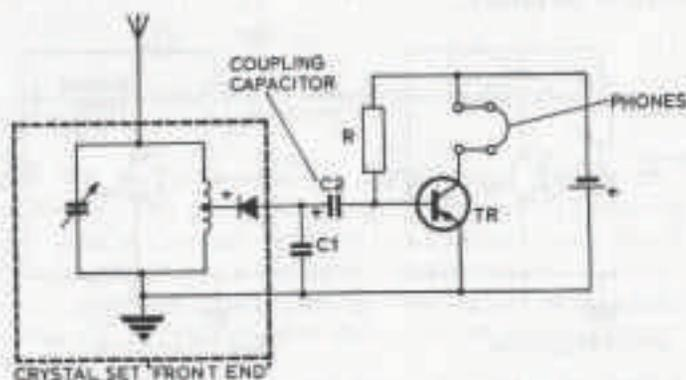
Fig. 5.2 Circuit 5. Crystal set with single stage of amplification. Any BF transistor can be used for TR.
