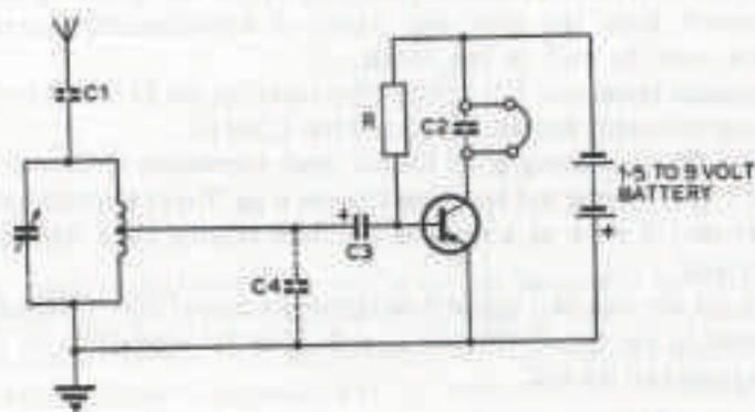
Fig. 3.7 *Circuit 3.* Crystal set with amplification.
