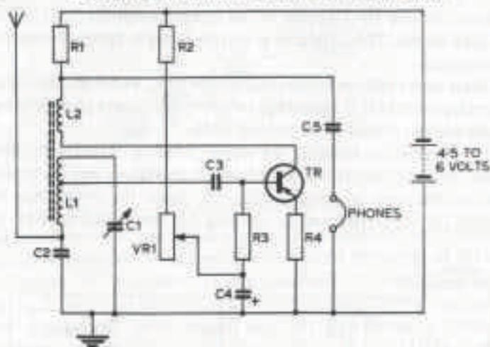
Fig. 9.10 *Circuit 21.* 'Mighty Atom' single-transistor receiver. This particular circuit design is by Weyrad, matching one of their special regen aerial coils. It is a regenerative receiver which uses a minimum of components and is capable of excellent performance for such a simple circuit. Matching phones are 50-100  $\Omega$ .
