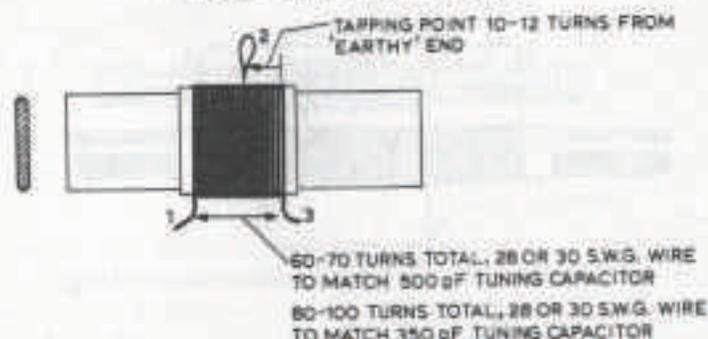
Fig. 4.6 Medium-wave winding for a ferrite slab.
