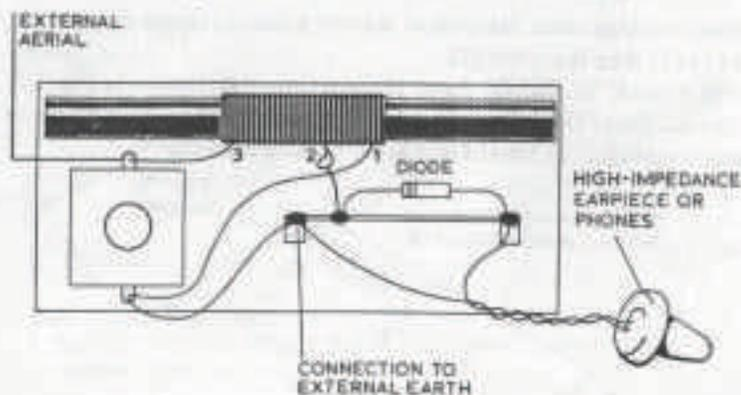
Fig. 3.4 Wiring connections to complete the crystal set.
