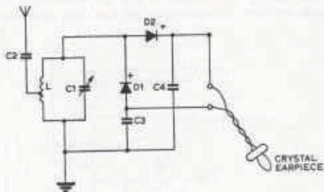
Fig. 3.8 *Circuit 4.* Double diode crystal set.
