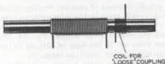
Fig. 4.9 'Loose' inductive coupling with separate coupling coil.
