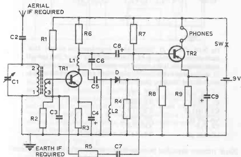
Fig. 9.9 *Circuit 20*. Four-stage reflex receiver. This is an extended version of the design given in Fig. 9.6—the same basic circuit with the addition of an AF amplifier stage. Using low-power transistors, output power is matched to high-impedance phones.
