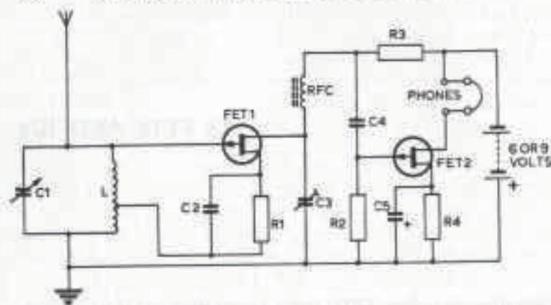
Fig. 13.2 Circuit 26. Simple regenerative receiver using P-channel FETs.
