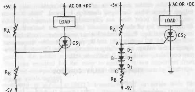
$R_A$ ,  $R_B$  - Thermistor and ref. resistor . . . approx. 2K at temp. set point.
