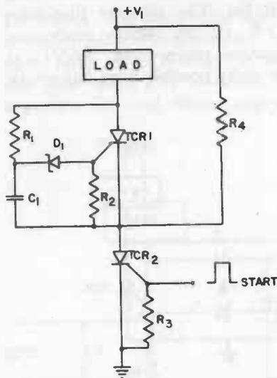
For  $V_1 = 50V$ , TCR2 is a 2N1595,  $R_3 = 1K$ , and  $R_4 = 5K$
