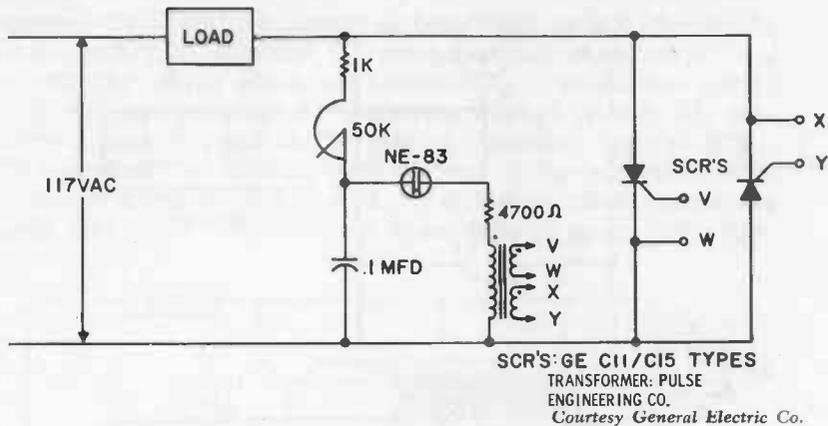
Phase-controlled trigger circuit.
