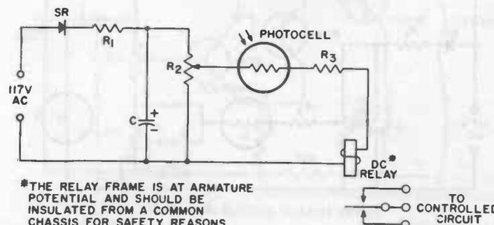
\*THE RELAY FRAME IS AT ARMATURE POTENTIAL AND SHOULD BE INSULATED FROM A COMMON CHASSIS FOR SAFETY REASONS.
