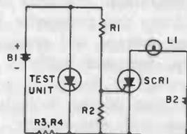
(E) Forward-leakage-current mode.
