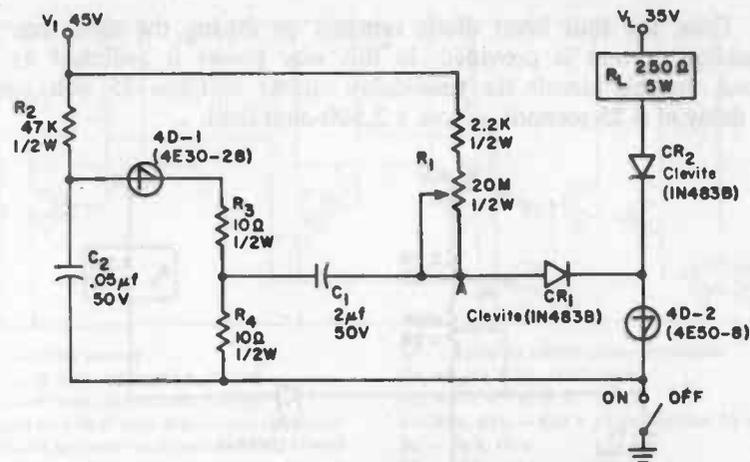
Courtesy Shockley Transistor, Unit Cleveite Transistor. Long time-delay circuit.
