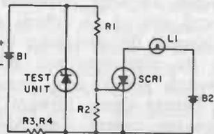
(D) Reverse-leakage-current mode.
