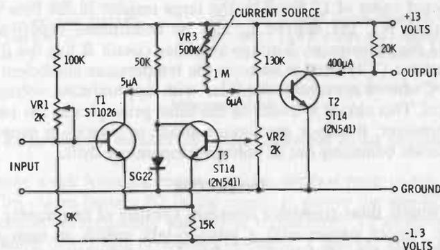
(B) Circuit with compensation for voltage drift.
