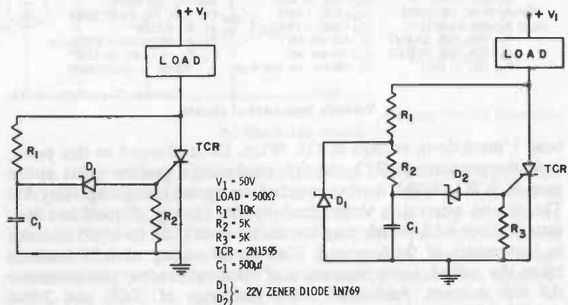
(A) Circuit with delay affected by supply voltage.
