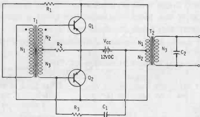
T<sub>1</sub> - Saturating feedback transformer
