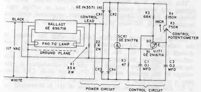
through CR4, C2, control potentiometer R5, R4, and CR1, charging C2. Simultaneously C1 is charged through R3. When the charge across C2 becomes sufficient to fire unijunction transistor UJT1, C2 discharges through UJT1 and resistor R2 producing a pulse at the gate of controlled rectifier SCR1. SCR1 now conducts for the remainder of the positive half cycle passing current to the fluorescent lamp. At the end of the positive half cycle, the voltage across SCR1 drops to zero and it switches off.
