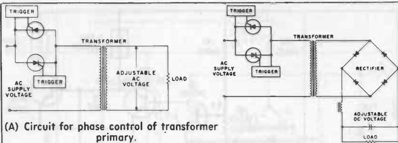
(A) Circuit for phase control of transformer primary.
