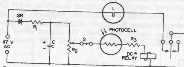
\* THE RELAY FRAME IS AT ARMATURE POTENTIAL AND SHOULD BE INSULATED FROM A COMMON CHASSIS FOR SAFETY REASONS.
