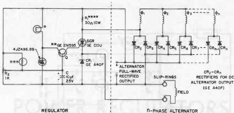
\*USE A GE NO. 428 LAMP HERE IF THE ALTERNATOR IS DESIGNED TO SELF-FLASH FROM RESIDUAL OUTPUT.
