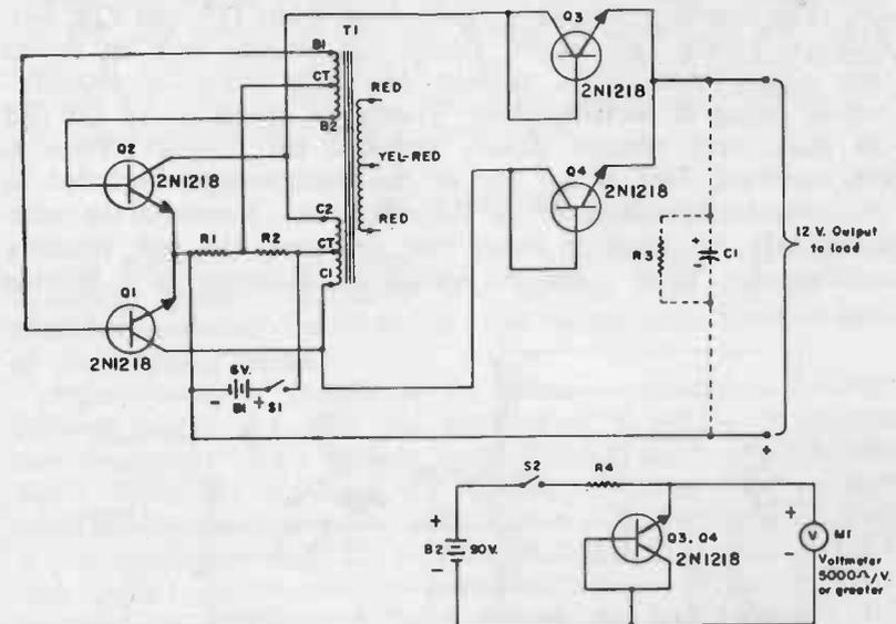
Test of inverse voltage for diode configuration of Q3 & Q4. Voltmeter should read 20 Volts or greater.
