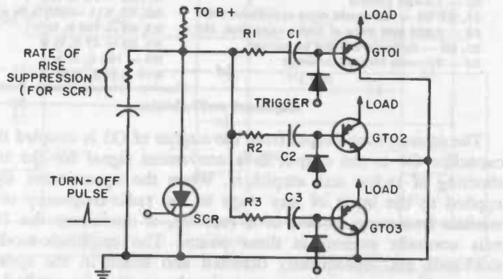
(B) Circuit using several gated turn-off switches.
