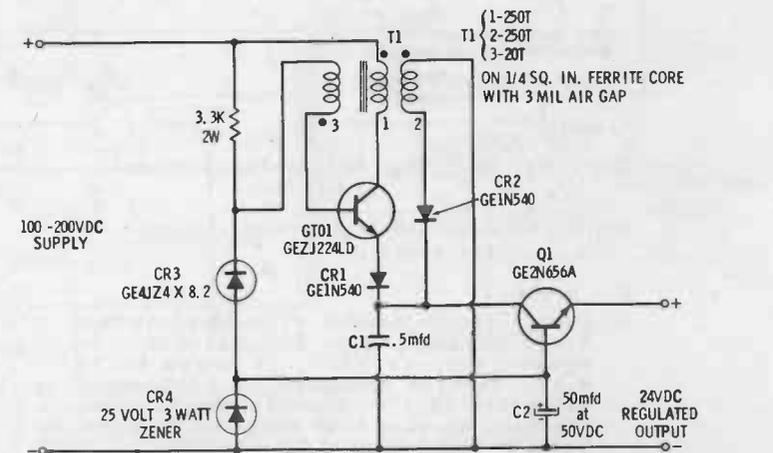
Circuit for 200VDC to 24VDC converter.
