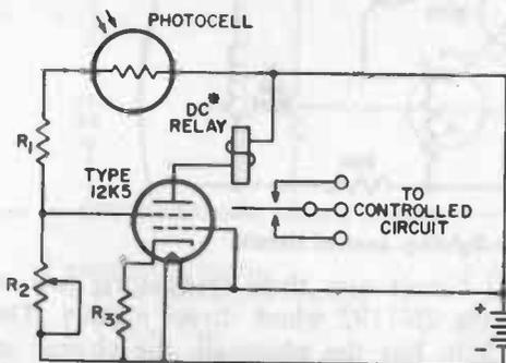
(C) Circuit with vacuum-tube amplifier.
