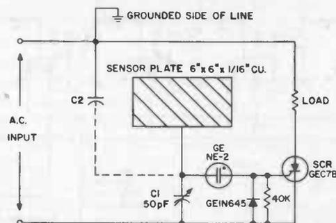
NOTES: (1) C2 IS EQUIVALENT CAPACITY OF SENSOR PLATE W.R.T. GROUND.
