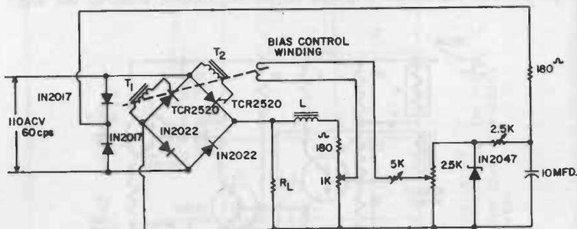
T<sub>1</sub>, T<sub>2</sub>—Magnetics Inc. Type 4181-001—FULL WAVE MAGNETIC CONTROL
