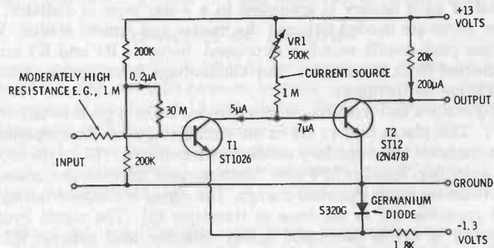
(C) Circuit with compensation for current drift and approximate compensation for voltage drift.
