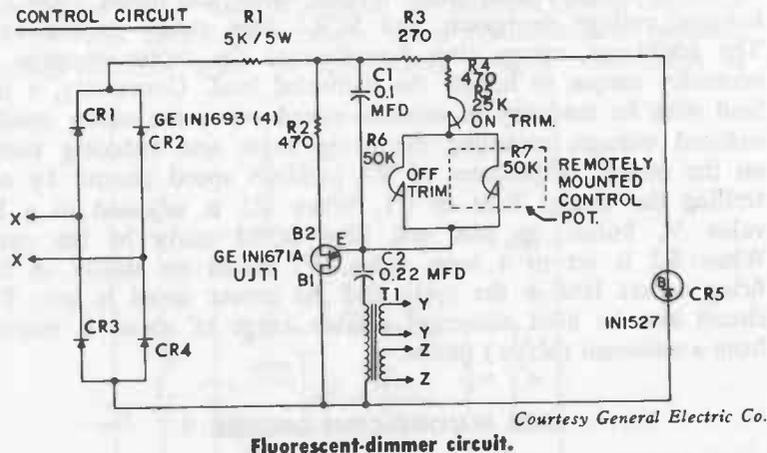
sates for line voltage changes over a half-cycle of line frequency by advancing the SCR firing angle when the line voltage drops. It retards the firing angle when the voltage rises. This feature is particularly desirable when the dimmer is operated from power lines subject to voltage regulation.
