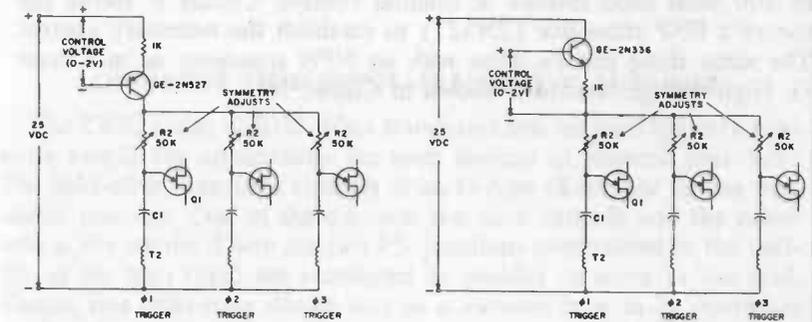
(F) PNP-transistor control circuit.
