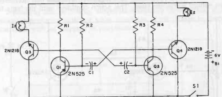
$$\begin{aligned} \text{On time Lamp I1} &= 0.69 R_3 C_2 \\ \text{or Off time Lamp I2} &= 0.69 R_3 C_2 \\ \text{On time Lamp I2} &= 0.69 R_2 C_1 \\ \text{or Off time Lamp I1} &= 0.69 R_2 C_1 \end{aligned}$$
