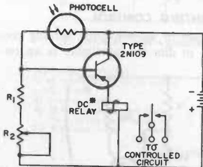
(B) Circuit with transistor amplifier.
