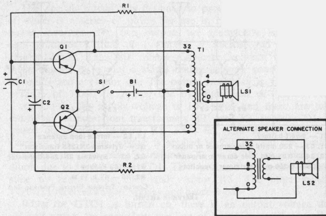
B1 — 12-volt battery (1 ampere drain) conventional auto or boat battery, or 2 Burgess F4P1 batteries wired in series.
