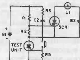
(C) Forward-voltage drop and gate-trigger mode.
