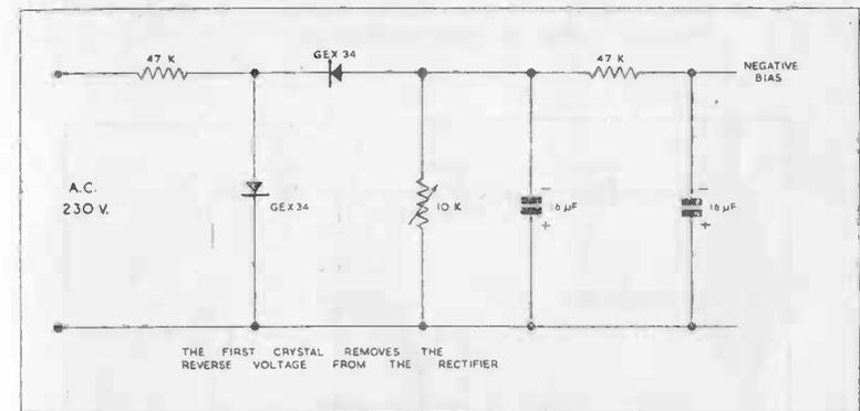
FIG. 17(a). VARIABLE BIAS SUPPLY. THE FIRST CRYSTAL REMOVES THE REVERSE VOLTAGE FROM THE RECTIFIER.
