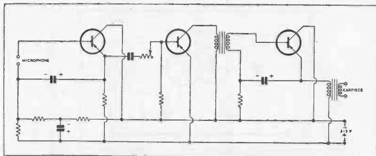
FIG. 39. CIRCUIT OF COMMERCIAL HEARING AID.
