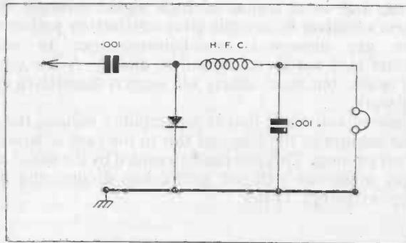
FIG. 18. SIGNAL TRACER.
