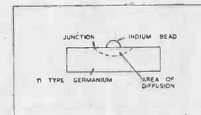
FIG. 3. MAKING AN ALLOY JUNCTION
