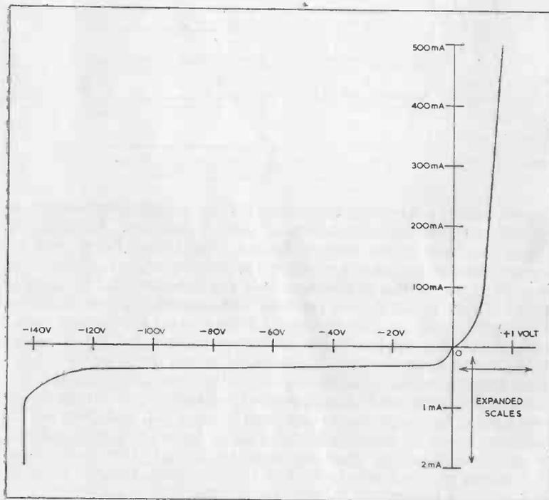
FIG. 4. CHARACTERISTIC CURVE OF A  $p-n$  JUNCTION DIODE.
