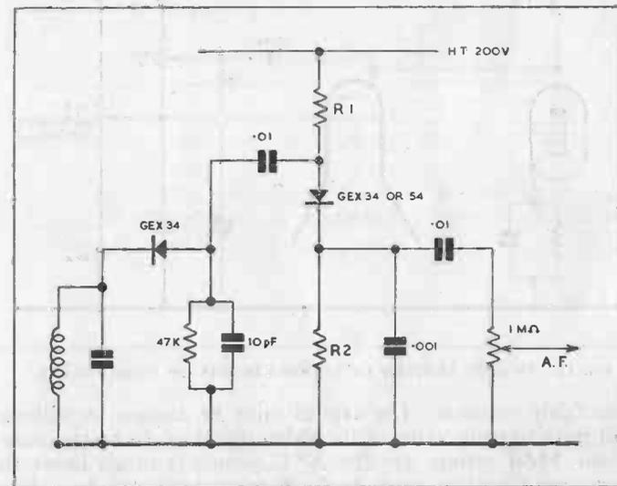
FIG. 11. TV SOUND DETECTION AND LIMITING.
