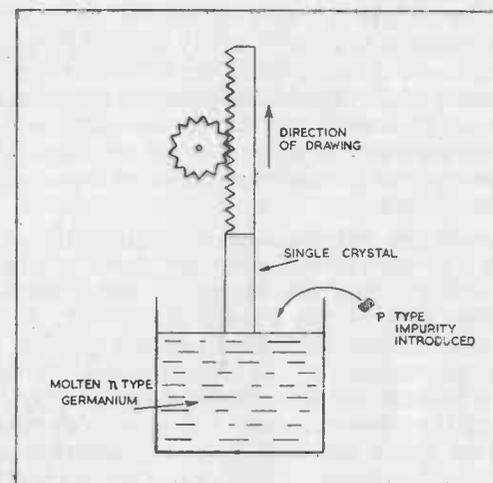
FIG. 2. MAKING A GROWN JUNCTION.
