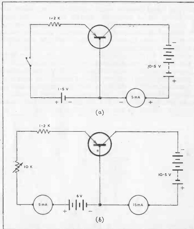
FIG. 43(a). CIRCUIT FOR ROUGH CHECK OF JUNCTION OR POINT-CONTACT TRANSISTORS.
