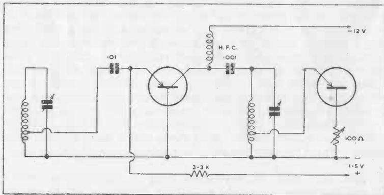
FIG. 25. POINT-CONTACT TRANSISTOR H.F. STAGE.
