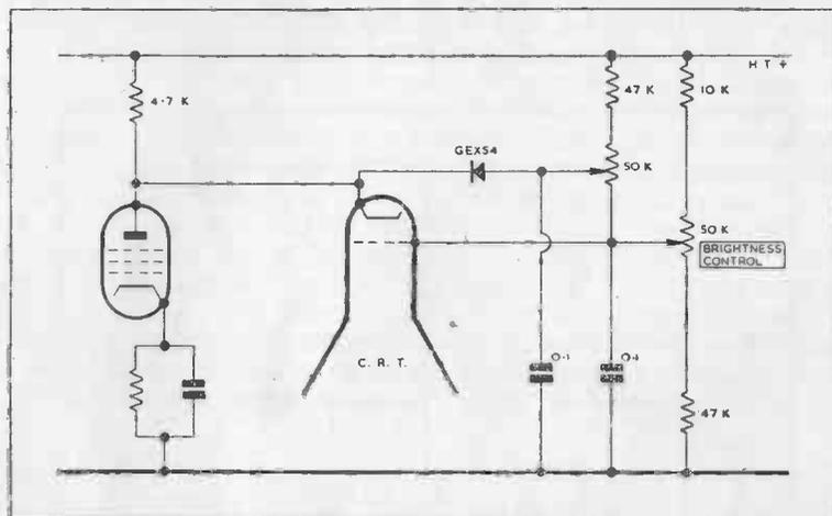
FIG. 12. TV SPOT LIMITER IN ANODE CIRCUIT OF VIDEO VALVE.
