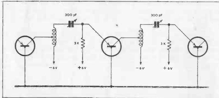
FIG. 33. SERIES-TUNED I.F. STAGE WITH JUNCTION TRANSISTORS.
