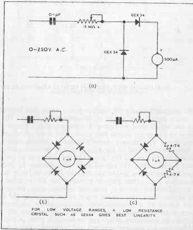
FIG. 18(a). SOME A.C. METER CIRCUITS. FOR LOW VOLTAGE RANGES A LOW RESISTANCE CRYSTAL (SUCH AS GEX 64) GIVES BEST LINEARITY.
