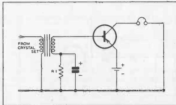
FIG. 35. TRANSFORMER COUPLED AMPLIFIER.
