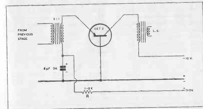
FIG. 20. POINT-CONTACT TRANSISTOR OUTPUT STAGE.
