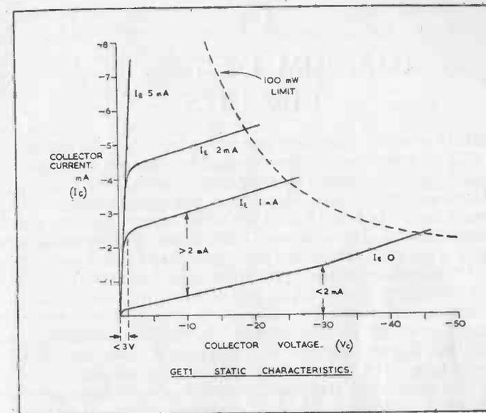
FIG. 9. COLLECTOR-CURRENT CURVES OF POINT-CONTACT TRANSISTOR.
