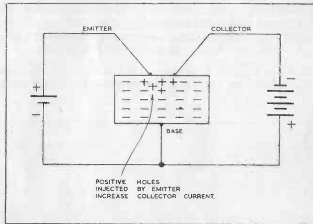
FIG. 8. SCHEMATIC ARRANGEMENT OF POINT-CONTACT TRANSISTOR.
