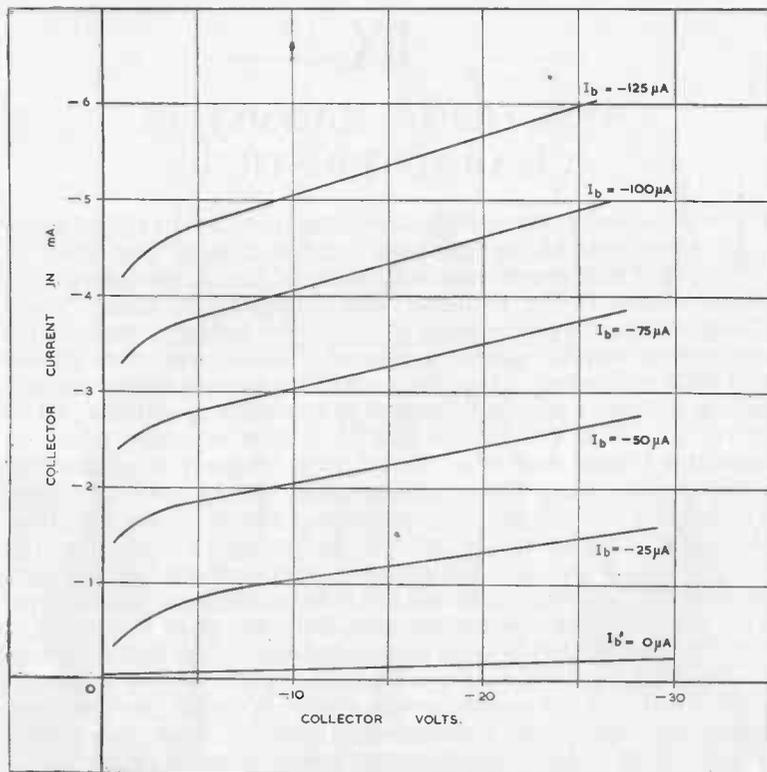
FIG. 32. COLLECTOR-CURRENT CURVES OF A TYPICAL *p-n-p* JUNCTION TRANSISTOR IN EARTHED-EMITTER CONNECTION.
