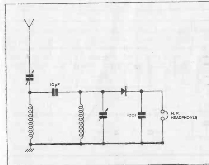
FIG. 16. TWO-CIRCUIT CRYSTAL RECEIVER.
