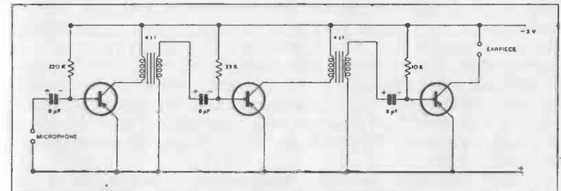
FIG. 38. FUNDAMENTAL CIRCUIT OF HEARING AID AMPLIFIER.
