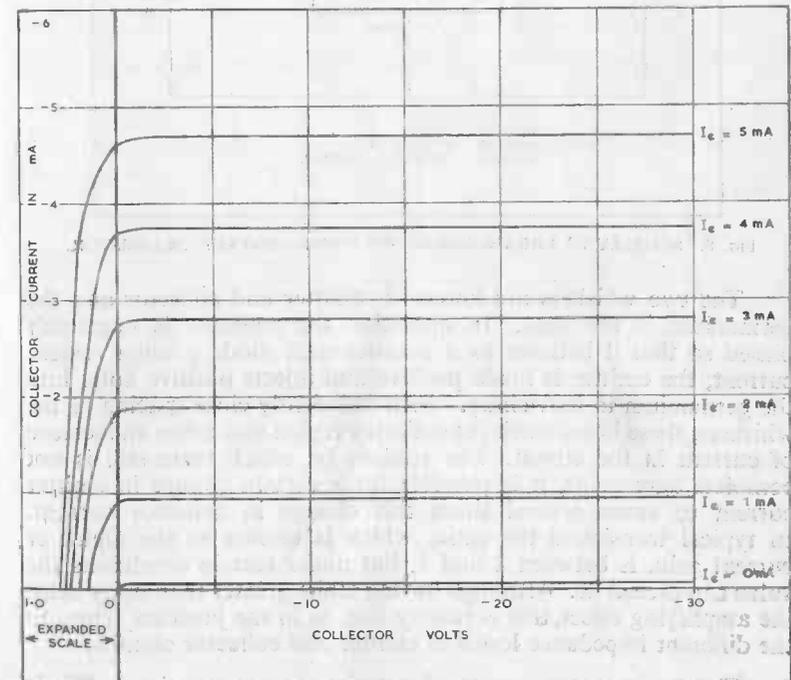
FIG. 7. COLLECTOR-CURRENT CURVES OF A TYPICAL  $p-n-p$  JUNCTION TRANSISTOR OF  $\alpha = .95$  APPROX.
