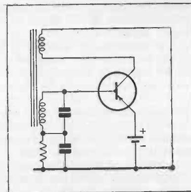
FIG. 40. JUNCTION TRANSISTOR L.F. OSCILLATOR.
