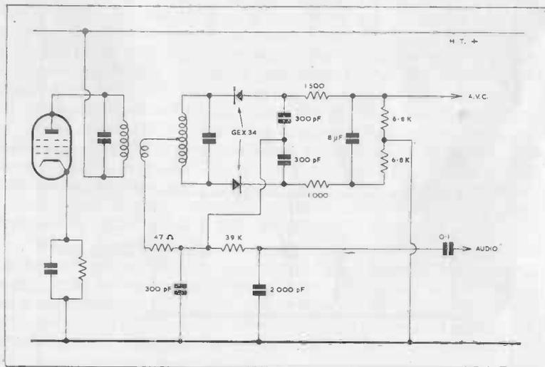
FIG. 17. RATIO DETECTOR USING CRYSTAL DIODES.
