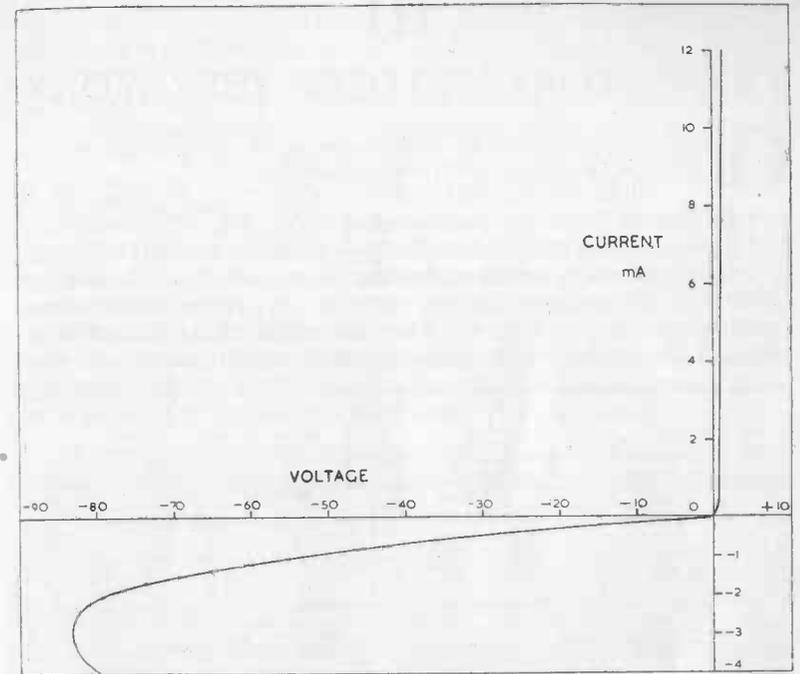
FIG. 5. CHARACTERISTIC CURVE OF A TYPICAL POINT-CONTACT GERMANIUM DIODE.
