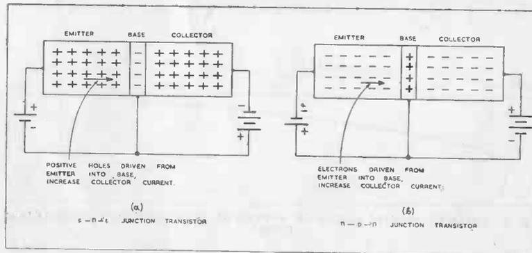
FIG. 6. (a)  $p-n-p$  JUNCTION TRANSISTOR. (b)  $n-p-n$  JUNCTION TRANSISTOR.
