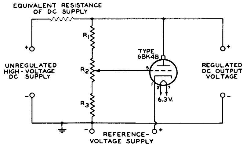
Typical performance data for this basic circuit with certain characteristics of the unregulated dc supply and related voltage-divider values are given in the tabulated data. Other combinations are feasible within the maximum ratings and the maximum circuit values for the 6BK4B.
