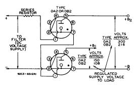
Typical circuit using two OA2's or two OB2's to provide regulated supply voltages of approximately 300 or 216 volts and 150 or 108 volts to load. Socket connections are so made that voltage on load is removed when either tube is taken from its socket.
