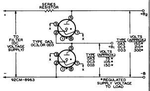
Typical circuit using two 0A3's, two 0C3's, or two 0D3's to provide regulated supply voltages of approximately 150, 210; or 300 volts and 75, 105, or 150 volts to load. Socket connections are so made that voltage on load is removed when either tube is taken from its socket.
