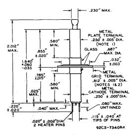
NOTE I: MAXIMUM ECCENTRICITY OF CENTER LINE (AXIS) OF PLATE TERMINAL OR GRID-TERMINAL FLANGE WITH RESPECT TO THE CENTER LINE (AXIS) OF THE CATHODE TERMINAL IS 0.010".
